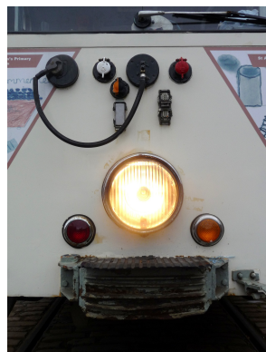
Detail from 392. L to R: indicators, front connect points, emergency stop.
